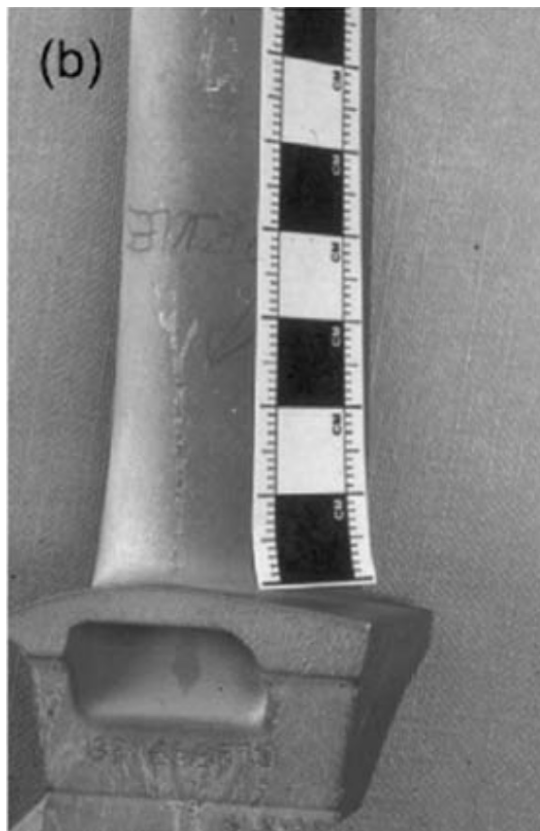
Figure 2.14: Freckle chain defects in directionally solidified superalloys [6].
