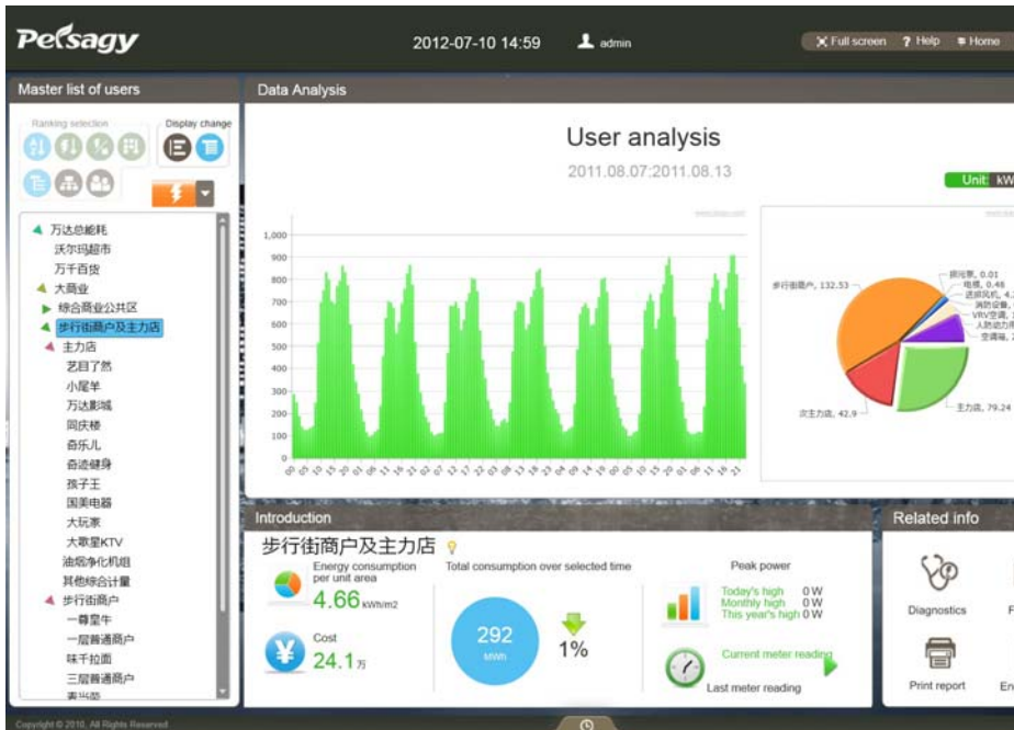
(a) Tenant comparison, showing end-use energy and daily use tracking.
