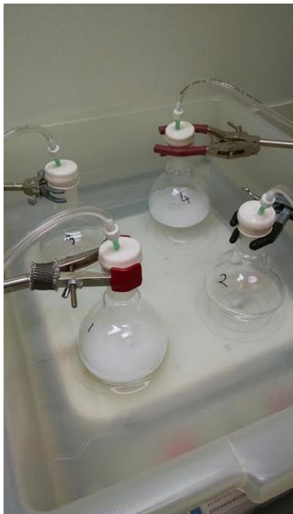
CBMA synthesis (precipitate forming) done under nitrogen protection.
