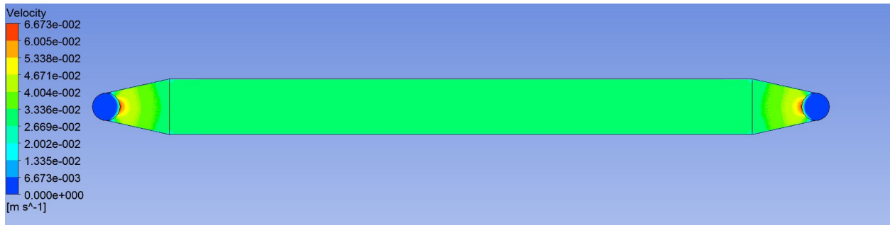
Figure 3.3: ANSYS simulation showing fully developed flow before substrates are reached, and uniform velocity across the length and width of the channel.
