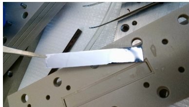
Figure 5.11: Disassembly of PEEK flow cell after 2-hour blood flow at a shear rate of 1000/s. There were some presence of white platelet clots on the flow path.
