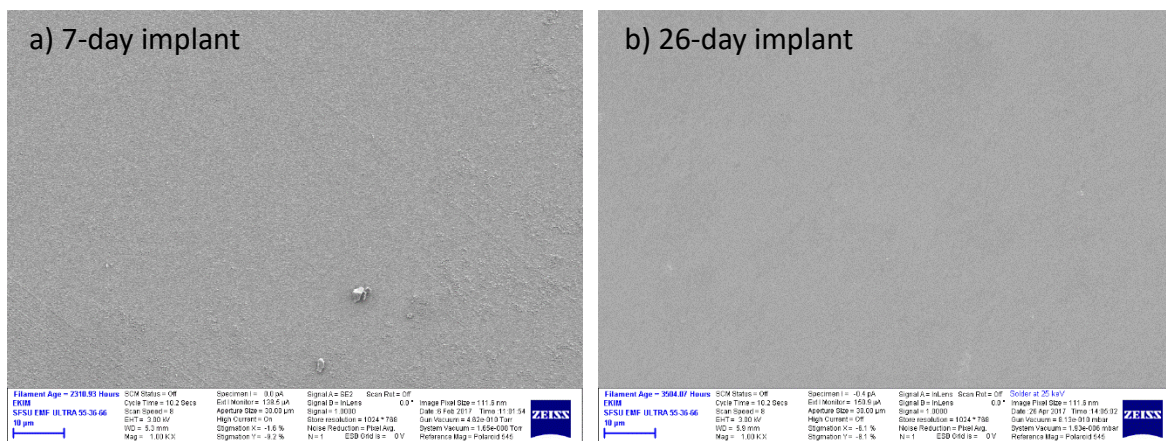
Figure 6.8: Representative SEM images of the pSBMA-silicon surfaces following (a) 7-day and (b) 26-day implant.
