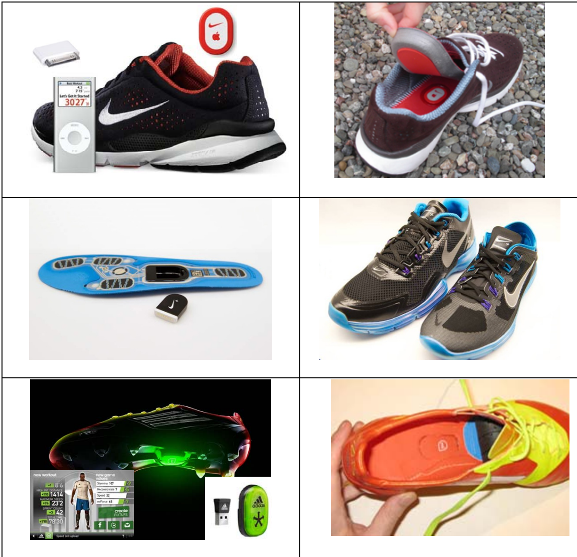
Figure 16. Nike+ iPod (old and new versions) and Adidas Speed_Cell systems; note that the transmitter is placed in a hollowed out space in the sole of a compatible shoe in both cases. The last two systems detect activities such as shuffling, stepping, lunging and jumping.
