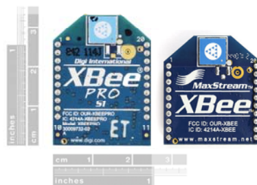
Figure 9. Dimensions of XBee Pro and XBee wireless modules.
