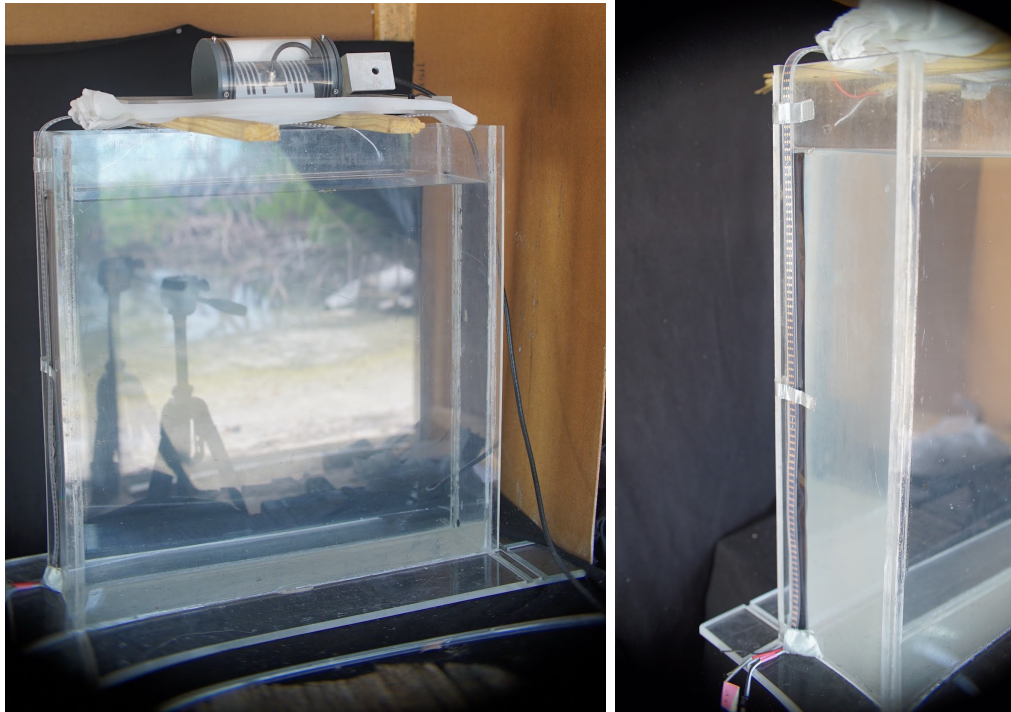
Figure C.1: Experimental set-up for dichotomous choice assays of female behaviors. (A; left) tank filled with seawater. On the top of the tank is a large infrared LED light source, suspended above the water line. In between the water line and the light are two folded paint strainers to diffuse the directionality of the light. (B; right). Close-up on the LED light strips used to provide stimuli to single females in the tank. On both left and right sides were single tracks of LEDs controlled by Arduino and loaded with custom-written programs to stimulate displays. Black cloth is used to enhance contrast behind the transparent tank. Set-up as in Belize, but differs slightly in practice from set-up in Panama for logistical reasons.
