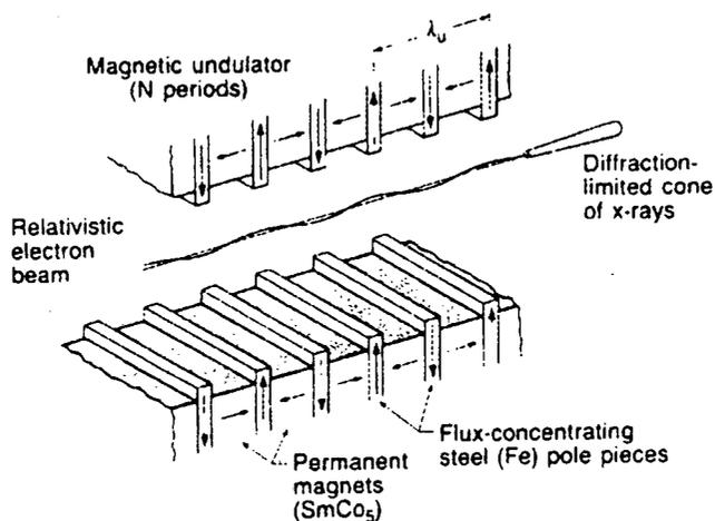
FIG. 2. Schematic drawing of a periodic magnet structure (an undulator) of period  $\lambda_u$  and with a number of periods,  $N$ . The oscillations of the electron beam passing through the structure produce ultraviolet and soft x-ray radiation (photons) of high spectral brightness.
