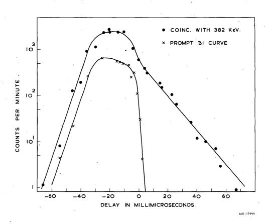
Fig. 1 Coincidence delay spectrum of the  $382~\rm kev$  gamma ray taken with the KX rays and higher energy radiation, detected in a 1 1/2" dia x 1" NaI crystals
