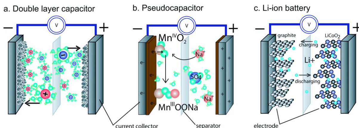
Figure 1.4. Basic mechanistic schematic for (a) double layer capacitor, (b) a pseudo-capacitor and (c) a lithium ion battery. 6
