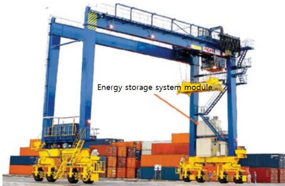
Fig. 1.12 Hybrid diesel/electric rubber tired gantry crane with an electrochemical capacitor energy storage system. 5
