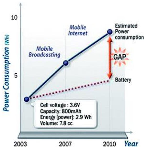
Figure 1.1. Comparison of the increase of power required for mobile electronic devices and the actual increase of battery power. 1
