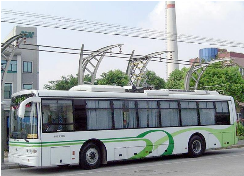
Fig 1.14. A bus that runs entirely on supercapacitors charges up at a bus stop in Shanghai. 17
