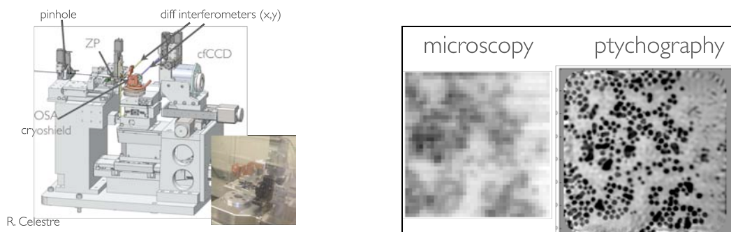
(left) The Nanosurveyor instrument with cryo-sample rotation stage and interferometer position sensing. (right) show the a STXM image and ptychographic reconstruction of a random aggregation of nanoparticles. The smallest visible features are 10 nm gold nanoparticles.
