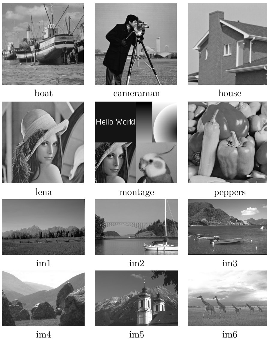
Figure 4.5: Test images for single image denoising. [Top] standard images of size 256 \times 256 ; [Bottom] natural images of size 481 \times 321 [2]
