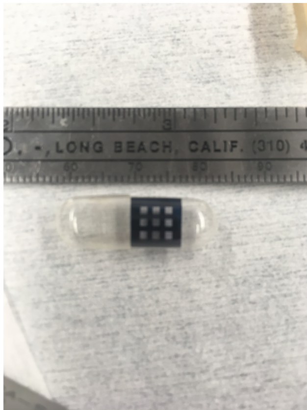
Figure 7.1: X-Ray transparent SiN windows used for the beamtime experiments to acquire the TR-XMCD signal in a\text{-Gd}_{10}\text{Tb}_{12}\text{Co}_{78} .
