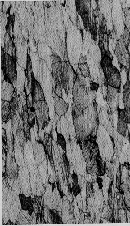
Plate 1. Thin sections of marble, Yule Creek, Colo. Transmitted polarized light. Lamellar structures are twins on [02\bar{2}1] plane.
