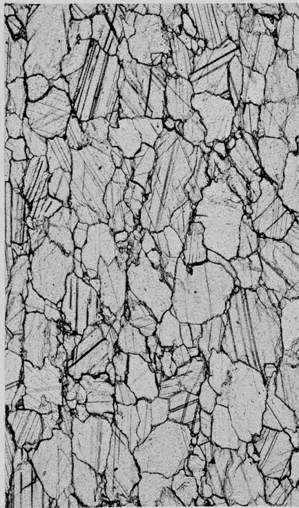
Plate 1. Thin sections of marble, Yule Creek, Colo. Transmitted polarized light. Lamellar structures are twins on [02\bar{2}1] plane.
