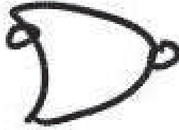
Figure 6.1: This example shows two different gates, the notbubble on the input side of a nor gate. The grouping classifier has difficulty learning the difference between the notbubble that should be joined on the output side of the gate, and the notbubble on the input side that should not be joined to the gate.
