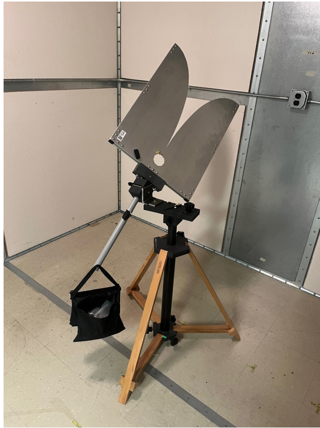
Figure 6.1: Picture of modified Com-Power antenna stand holding Vivaldi antenna for Run 1B. This antenna stand was designed for electromagnetic compliance applications and is non-conducting with the exception of a few pieces of metallic hardware.
