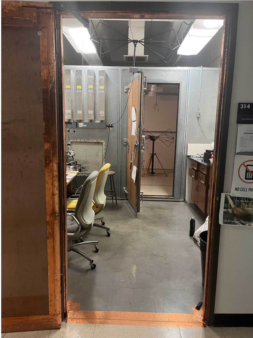
Figure 2.38: Photo of dark radio lab. The shielded room contains the main antenna as well as the LNA and power supply (not visible). The veto antenna can be seen hanging outside of the shielded room. The photograph was taken looking south.
