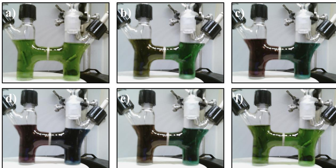
Figure 4.3. One full charge/discharge cycle of 3.2 , in \text{CH}_3\text{CN} with oxidation and reduction occurring in the left and right compartment on charging, respectively. (a-d) were taken during charging, and (e-f) were taken during discharging. (a) = ~0% state of charge (SOC), (b) = ~25% SOC, (c) = 50% SOC, (d) ~75% SOC, (e) ~35% SOC, (f) = ~0% SOC.
