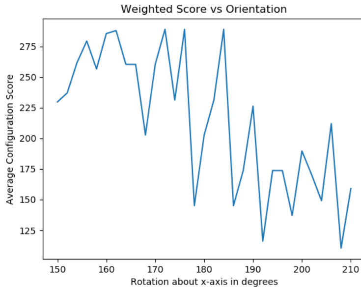
Figure 6.4. The average weighted configuration scores for a single target on the anterior surface of the chest at various needle \alpha -orientations. 180^\circ corresponds to the negative z-axis of the needle aligned perpendicular to the CT bed, representing a 90^\circ rotation from the original needle z-axis orientation.
