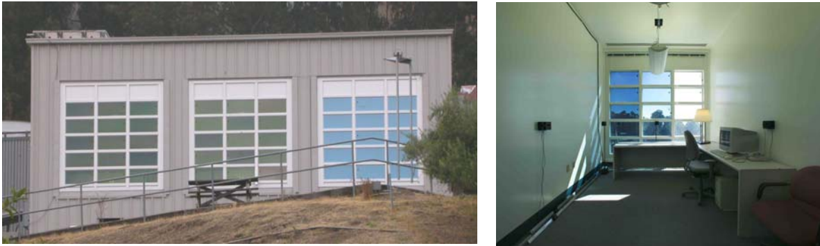
Figure 3. Exterior (left) and interior (right) view of the installed electrochromic windows. The two test rooms on the left in the exterior view are the EC windows and the single test room on the right is the reference room.
