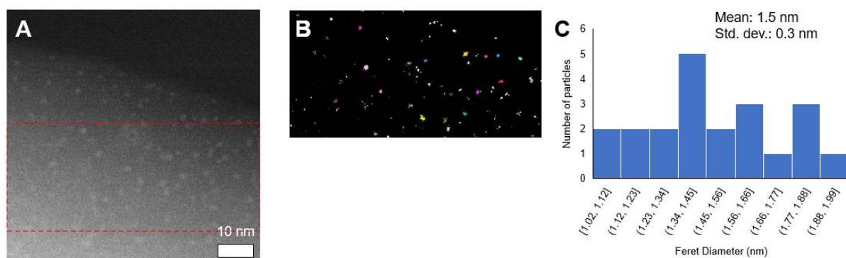
Figure S9. (A) HAADF-STEM Image 4 of 4-h-aged Cu-CHA. (B) Processed image data of Image 4 of 4-h-aged Cu-CHA showing clusters identified by automated analysis as different colors. (C) Histogram of the Feret diameters of clusters detected in (B). No outliers were identified in this analysis.
