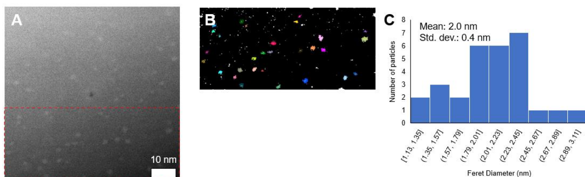
Figure S8. (A) HAADF-STEM Image 3 of 4-h-aged Cu-CHA. (B) Processed image data of Image 3 of 4-h-aged Cu-CHA showing clusters identified by automated analysis as different colors. (C) Histogram of the Feret diameters of clusters detected in (B). No outliers were identified in this analysis.
