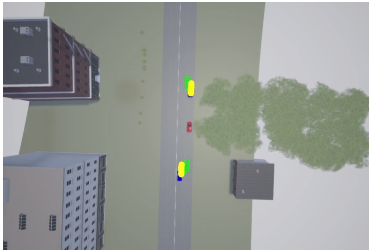
Figure 3.8: Drone view of the testing scenario including AV (red) and 2 TVs (blue) with predictions (yellow and green circles)
