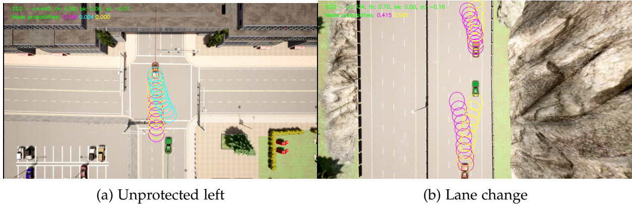
Figure 3.7: Carla simulation setup for unprotected left turn and lane change for AV (green) in the presence of TVs (orange) and multi-modal predictions (depicted by the ellipses). Code: https://github.com/shn66/SMPC_MMPreds
