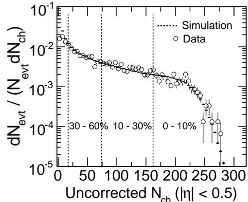
FIG. 3: Uncorrected charged particle multiplicity distribution (open circles) measured in the TPC within  $|\eta| < 0.5$  in Au + Au collisions at  $\sqrt{s_{NN}} = 9.2$  GeV. The dashed histogram represents the simulated multiplicity distribution. The vertical dashed lines reflect the centrality selection criteria used in the paper. Errors are statistical only.
