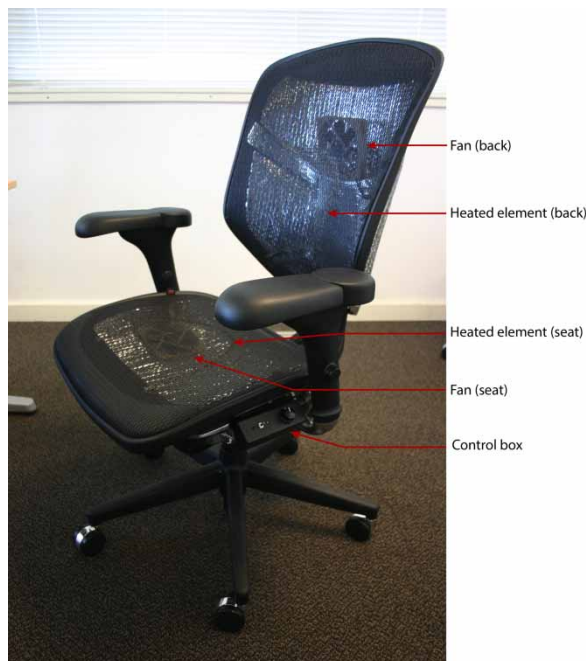
Figure 7 Personal Comfort System (PCS) heated and cooled chair. Source: Pasut et al. (2014)
