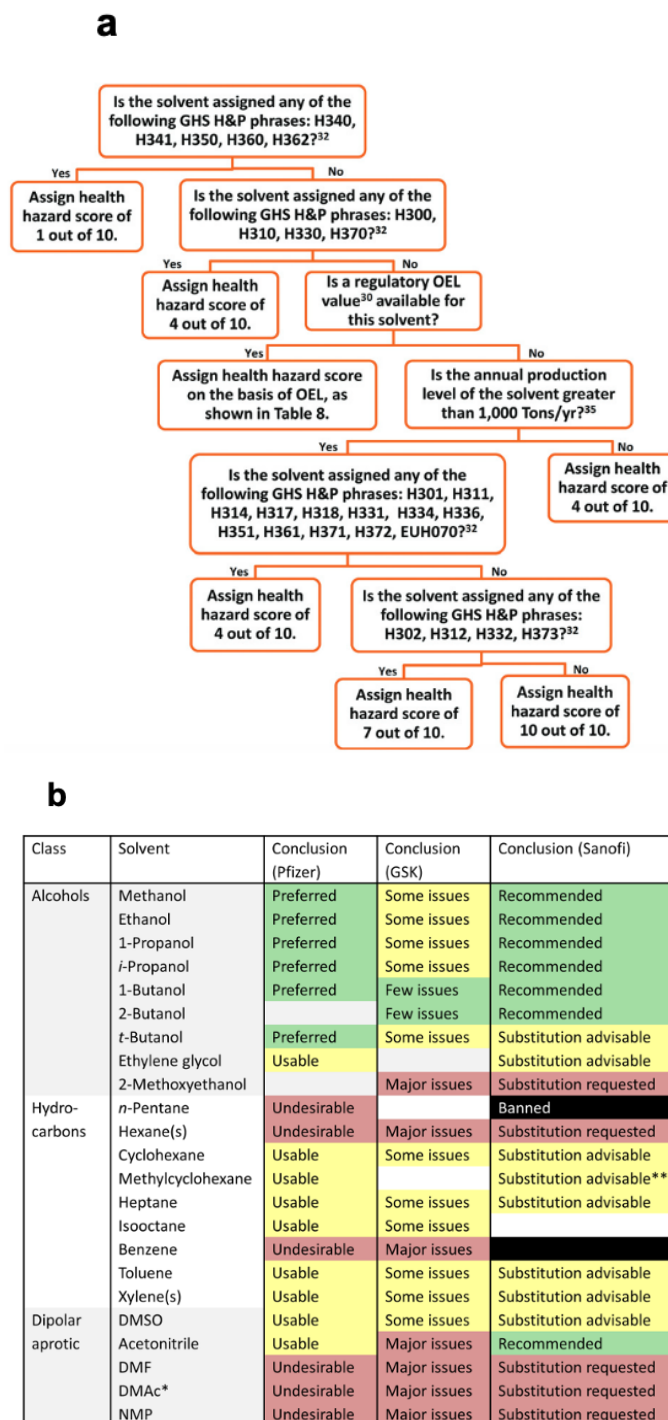
Figure 4.3: a) GSK decision tree for determination of GHS Hazard and Precautionary (H&P) phrases for a given solvent. b) Example classification of common solvents by different industry solvent rankings. Figure adapted from Alder et al. (2016) and Byrne et al. (2016) [133, 173].
