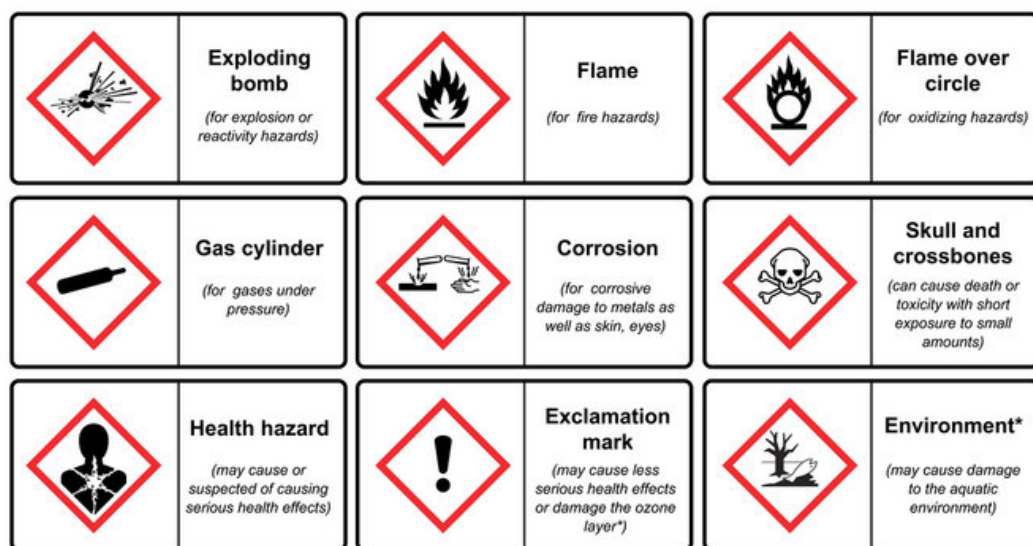
Figure 4.2: GHS pictograms used on labels to alert users of the chemical hazards to which they may be exposed. Each pictogram represents a distinct hazard.
