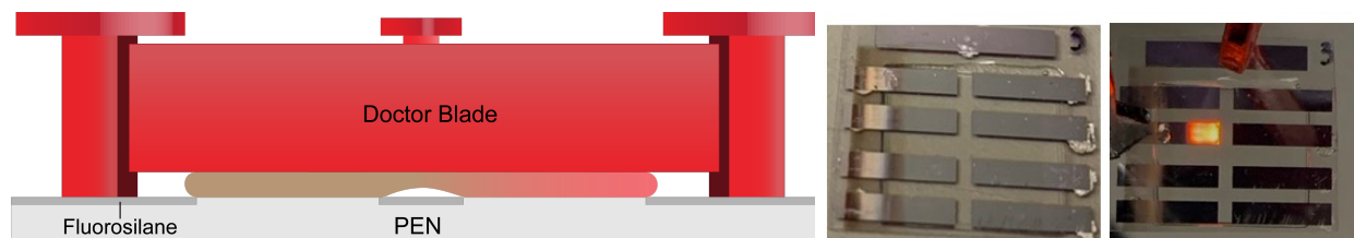
Figure 3.6: Illustration and images of merging effect on simultaneous printing. In this scenario, the OPD BHJ solution travels across the blade to the OLED side. Mixing with the OLED EML solution, the OPD BHJ solution leaves a streak of photoabsorbing along the edge of the OLED film, impacting the emissive area of the OLED. Dim emission of an OLED pixel is shown as a result as the OPD intermixing. The emission area is both smaller than intended and nonuniform.
