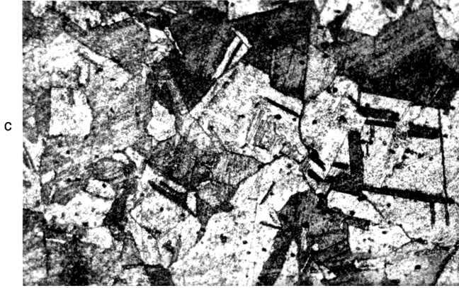
Plate 8.9. Metal microstructures (continued): (c) phase III, SF 5622, small piece of corroded metal, magnification 300 X, showing cold-worked and annealed microstructure; plate 8.2e; (d) phase IV, SF 3229, copper pin, magnification 240 X, showing cold-worked and annealed microstructure; figure 8.2c, plate 8.5a.
