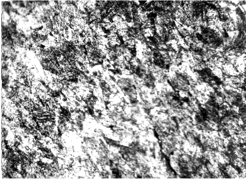
Plate 8.9. Metal microstructures (continued): (e) phase IV, SF 5625, piece of metal (bronze?), magnification 120 X, showing cold-worked microstructure; (f) phase Vb, SF 2084, lump of copper fragments, magnification 120 X, showing as-cast dendritic microstructure; (g) phase V, SF 5627, small piece of corroded copper, magnification 120 X, showing as-cast dendritic microstructure.
