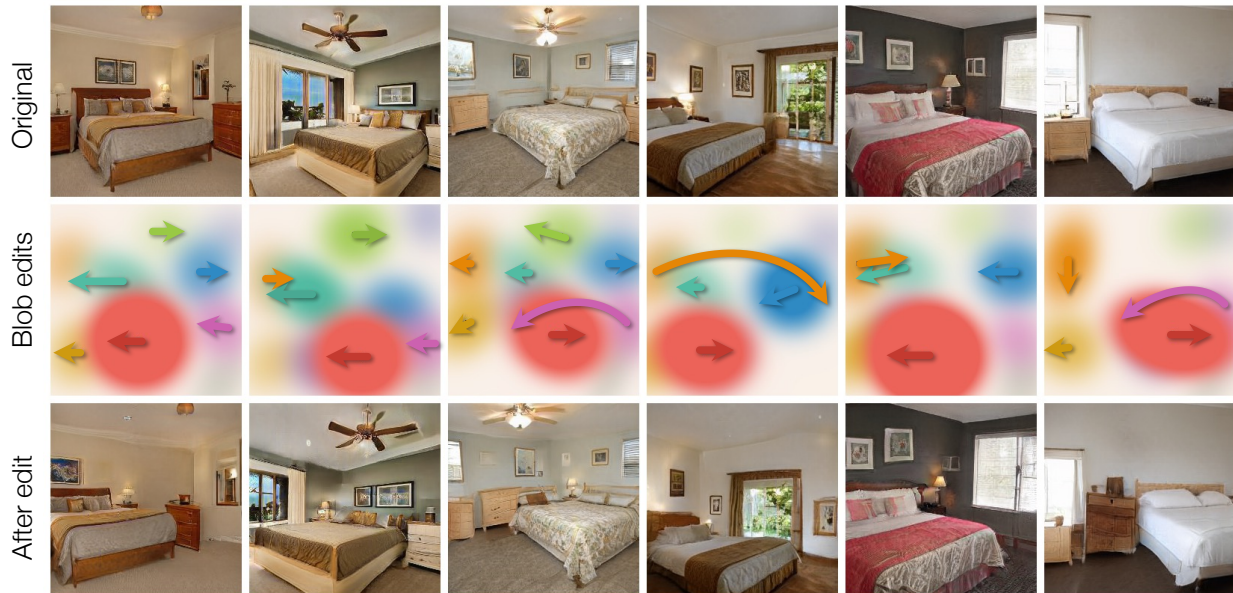
Figure 2.4: Moving blobs to rearrange objects: By modifying coordinates x_i of certain blobs as shown in the middle row, we can perform operations such as rearranging furniture in bedrooms. Note that since our representation is layered, we can model occlusions, such as the bed and the dresser in the leftmost and rightmost images.
