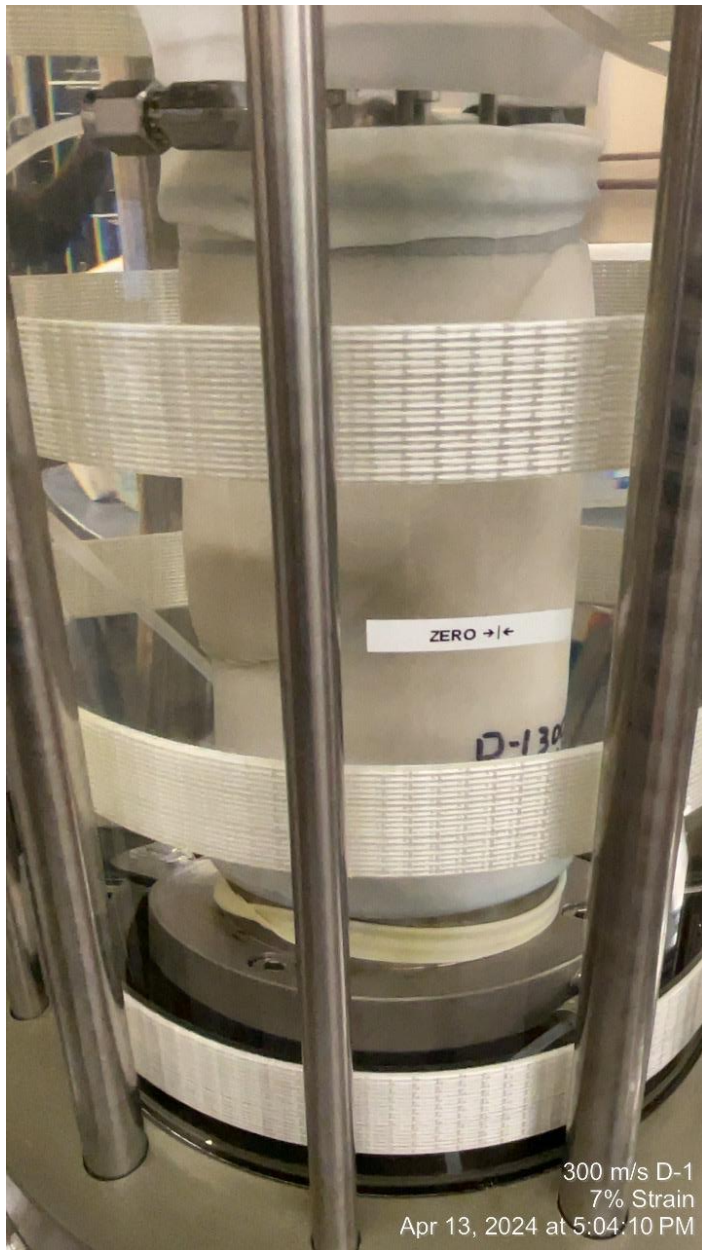
Figure 10. Shear band observed in 100S moderately cemented specimen at 7% strain.
