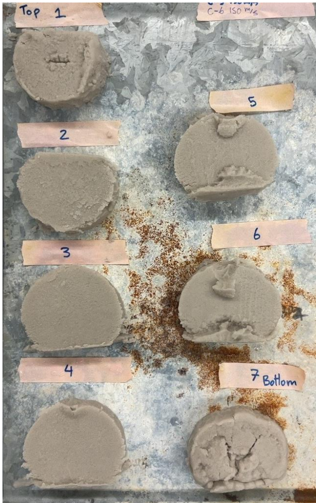
Figure 6. Specimen cut into segments for drying.
