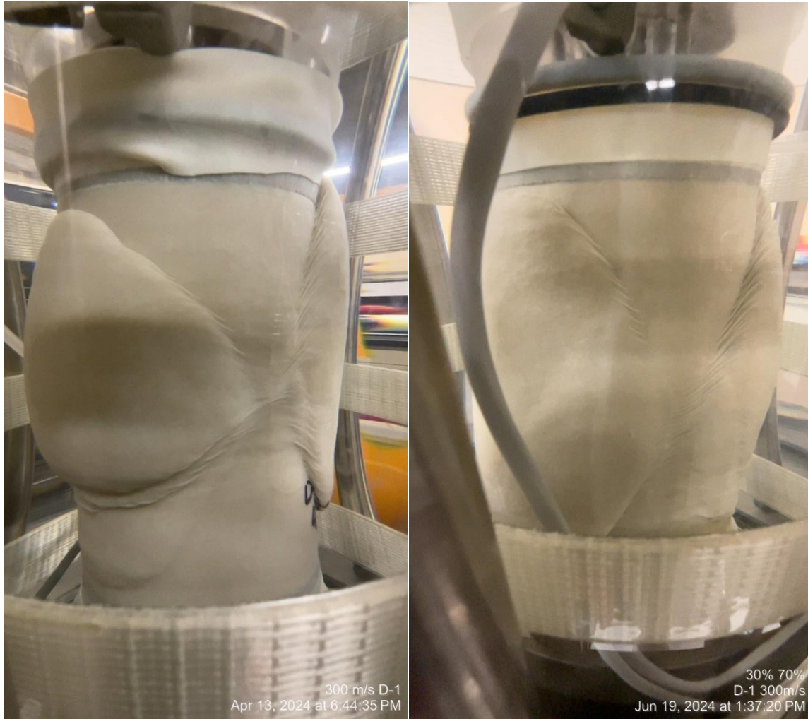
Figure 11. Shear band on loose 100S (left) and 70S30C (right) moderately cemented specimens.
