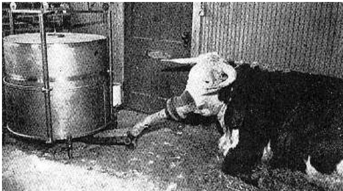
Figure 2. Face masks for respiration and methane emission measurements in the 1930's. Sourced from Washburn and Brody (1937).
