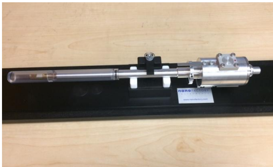
Figure 8.3 In situ TEM holder by Nanofactory capable of electrical bias
