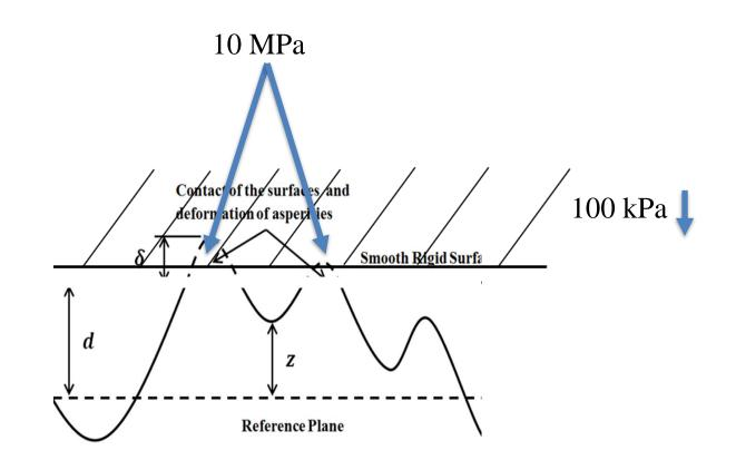
The load is carried by 1% of the surface (remainder not in contact) Yield strength controls contact structure and the maximum possible stress <sup>7</sup>
