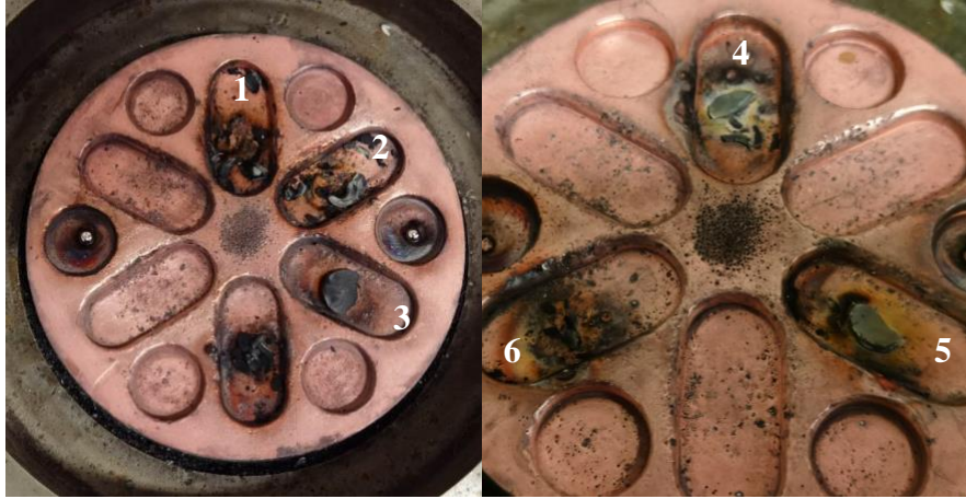
Figure 14. Arc Welded PDA coated Si Pellet via various power and time conditions: 1)75% power 3s; 2) 50% power 5s; 3) 50% power 3s; 4) 30% power 10s; 5) 75% power 3s; 6) 30% power 15s.
