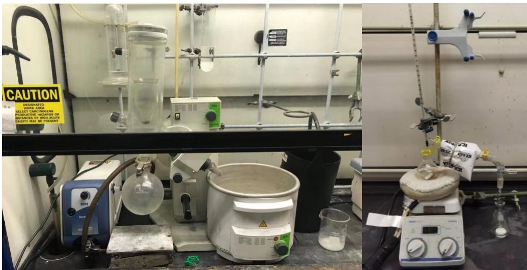
Figure 4. Experimental Set-up for Pickering Emulsion of SiMPs: Rotatory Evaporator (Left); Distillation Kit (Right)
