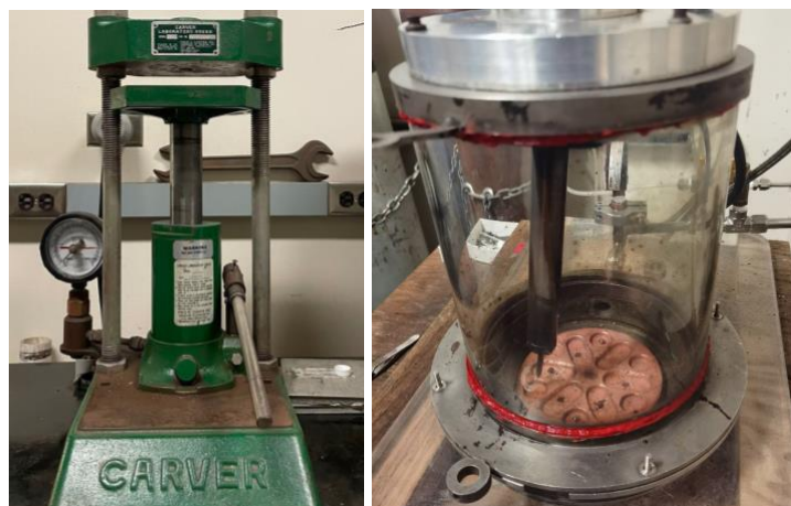
Figure 6. Experimental Set-up for Arc Welding: Hydraulic Press (left) and Home-made Arc Machine (right)
