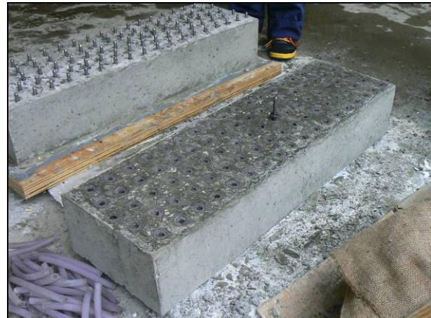
Figure 4.43: Demolded cast beam specimen.
