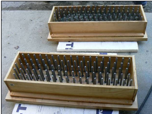
Figure 4.42: Cast beam specimen molds.
