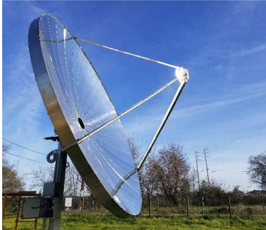
Figure 50: Two-axis tracking 7-m parabolic solar dish at the STEEL lab (UC Davis) in operation during an on-sun experiment with a prototype 8 cm x 8 cm micro-pin-array receiver.
