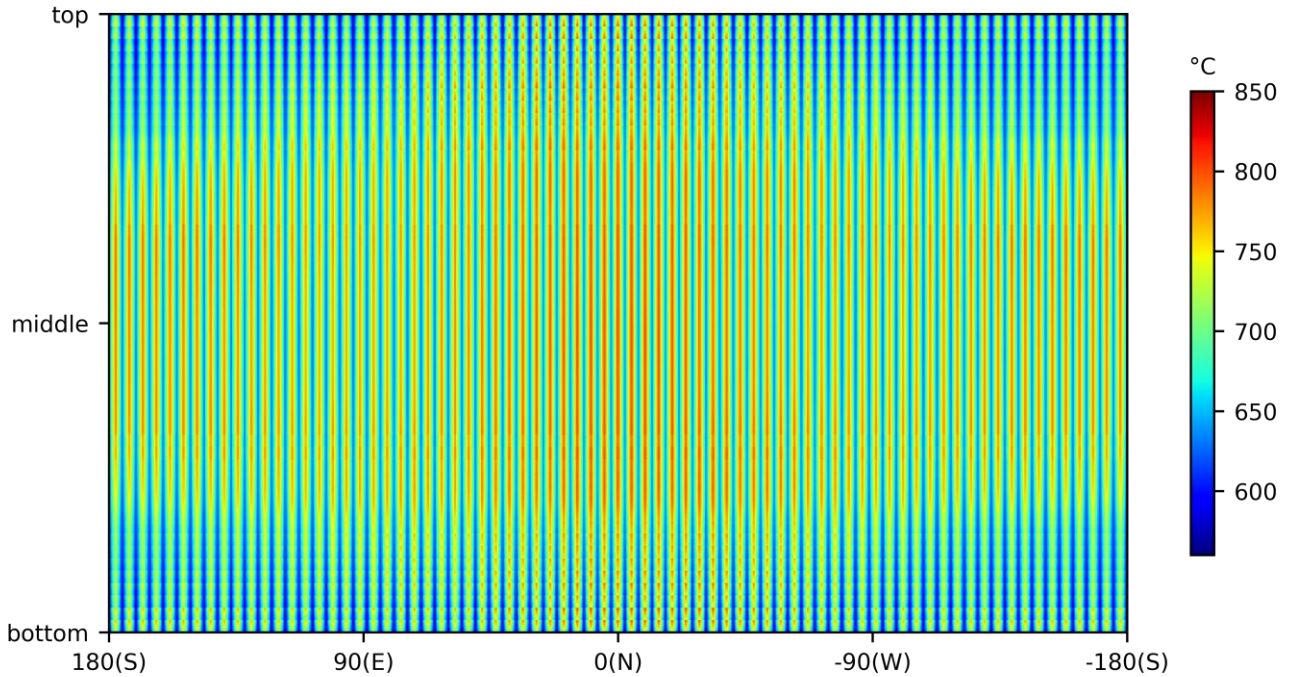
Figure 38: Surface temperature distribution over the receiver at solar noon on a hot summer day for the variable pin receiver.
