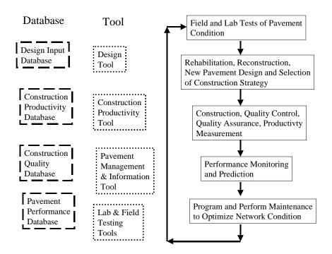
Figure 1. Interactions of tools and databases used to perform Caltrans pavement functions.
