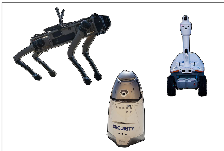
Figure 1.1: Some robot platforms that have been used for patrolling or urban search and rescue [31, 53, 94]. Example tasks include object inspection in unknown environments, collaborative mapping in harsh conditions, and patrolling a parking garage for parking infractions. Individual images grabbed from the google images search engine. The KnightScope [53] robot (bottom middle) in particular has been deployed in parking lots in San Bernardino County, CA and was recently authorized by the US government to operate in other parts of the country.
