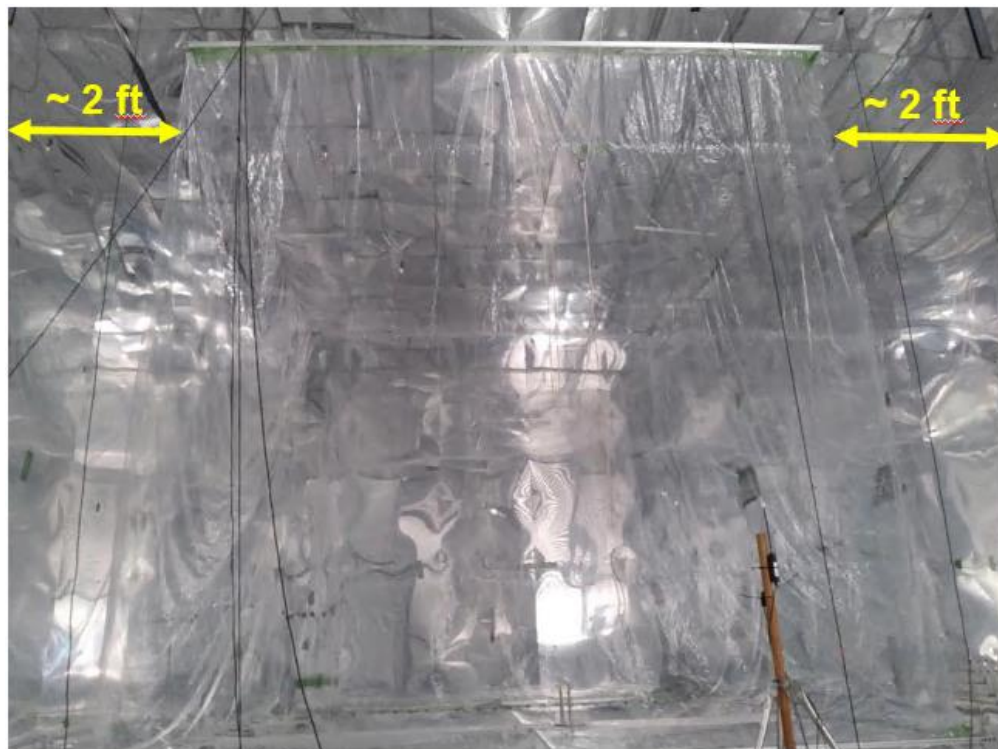
Figure 4-2. A picture of the real chamber. A distance of around 2 feet is kept between chamber walls and conductive aluminum enclosure walls.
