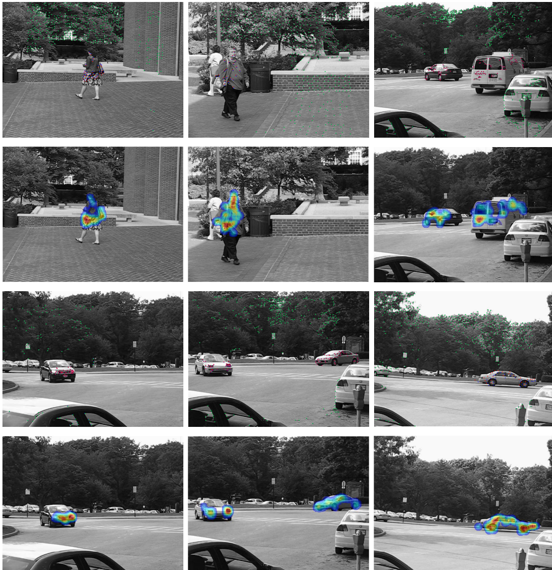
Figure 8.4: Sample results from the Hopkins 155 dataset: Odd rows: Images with tracked points. Red and green points show the locations of tracked points as predicted by the model. Points in green are the points that are classified as inliers and in red those that are classified as outliers. Blue dots (not visible for inlier points) are the true positions of tracked points. Even rows: Images showing in color the detected outliers. The color corresponds to a sum of Gaussians centered at each salient point.
