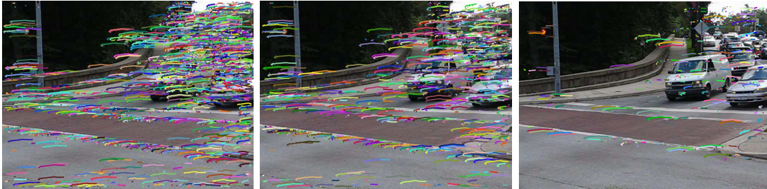
Figure 2.1: Varying the co-variant detection threshold produces different densities of trackable regions. There are typically three regions of interest, shown in the images. The tracks that persist through a wide a range of thresholds are typically the longest and most accurate.
