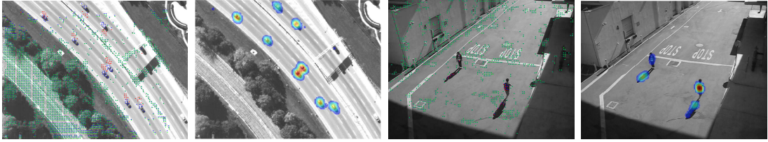
Figure 8.1: Detecting salient regions under camera motion: (1st, 3rd): Tracked feature points (blue) are classified as inliers (green) or outliers (red). (2nd, 4th): Estimated salient point density obtained by our algorithm.
