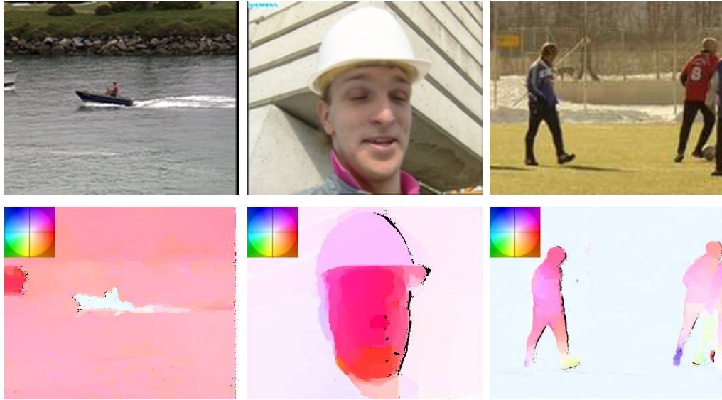
Figure 7.1: (COLOR) Occlusion detection and optical flow: Original images (top) and optical flow (bottom), visualized according to the color scheme shown in the top left corner of each image. Black regions are occluded, so no motion estimate is available since there is no region in image I(x, t - 1) that, transported with w(x, t) yields I(x, t) .
