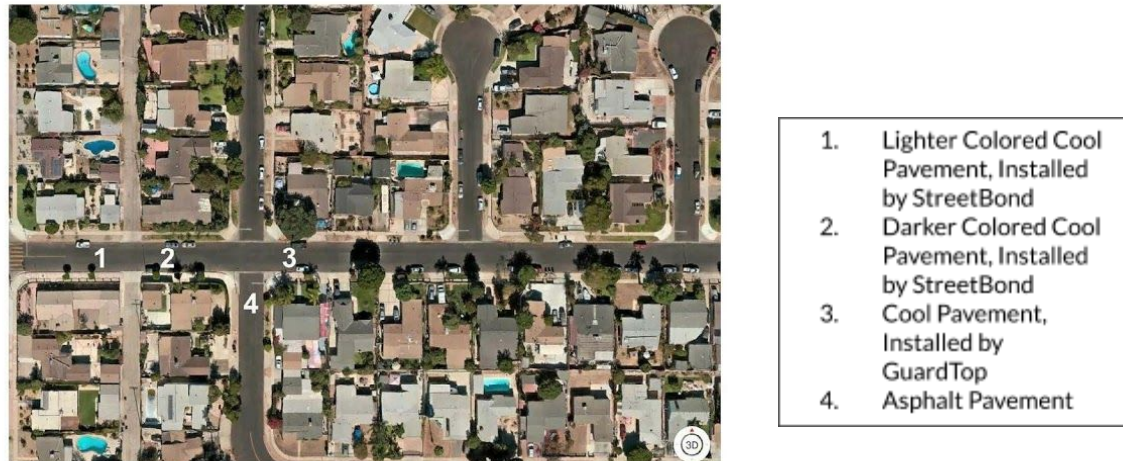
Figure 3- Location of the Kestrels Devices Placed on the Four Types of Surfaces
