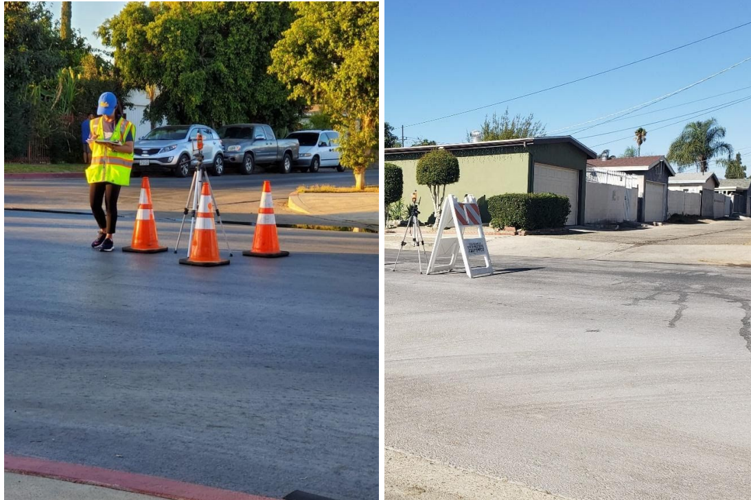
Figure 5 (a,b)- Kestrel Placed on Cool Paved Surface Installed by GaurdTop (left) and Lighter Colored Cool Surface Paved by StreetBond (right)
