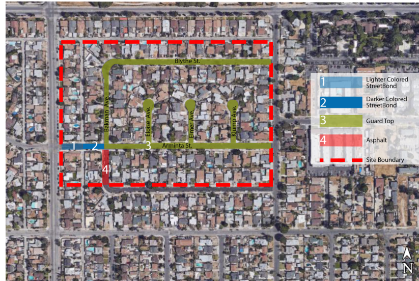
Figure 2- Study Area showing Locations of Cool Streets and the Asphalt Pavements
