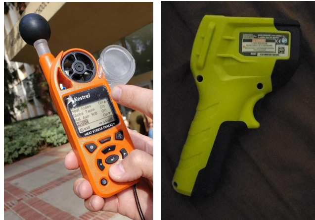
Figure 4 (a,b)- Heat Measurement Devices- Kestrel (left) and Heat Gun (right)
