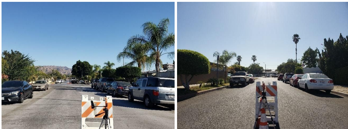
Figure 5 (c,d)- Kestrel Placed on Lighter Colored Cool Surface Paved by StreetBond (left) and on the Asphalt Top (right)
