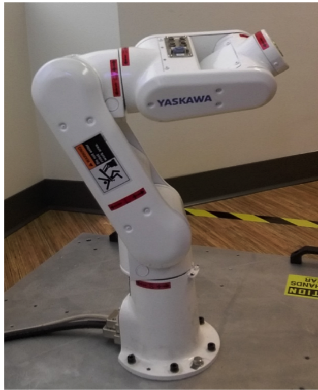
Figure 2.1: Yaskawa Motoman MHJ robot
