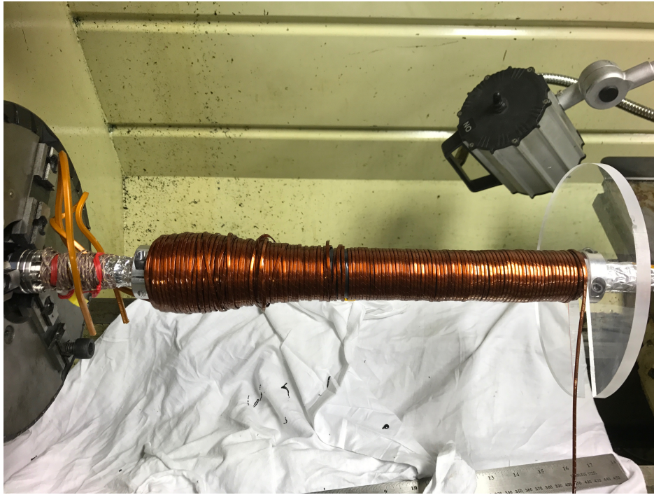
Figure 3.12: The long nipple was covered in tin foil and heating tape for vacuum baking purposes. A thermocouple was placed inside to monitor temperature. The magnetic wire was wound on a lathe.
