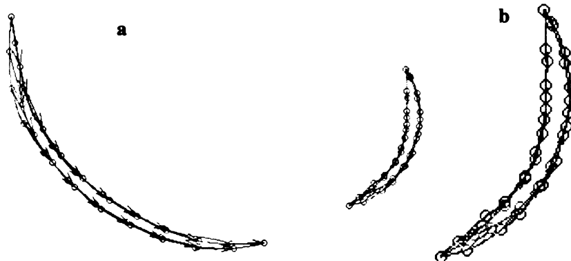
Fig. 4.4. (a) Artificial point matching of slice n (red) and slice n+1 (green). Corresponding points are indicated with small circles and connected with blue vectors. (b) Zoom of right segment of (a).
