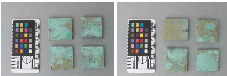
(e) P3 coupons after 24 hour immersion in 150 ppm Propolis 3 solution
