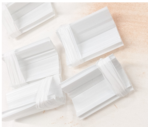
Figure A.23: Image detailing the individual coupons stands used during the artificial aging during the weight change experiments.
