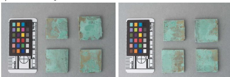
(c) P1 coupons after 24 hour immersion in 150 ppm Propolis 1 solution
