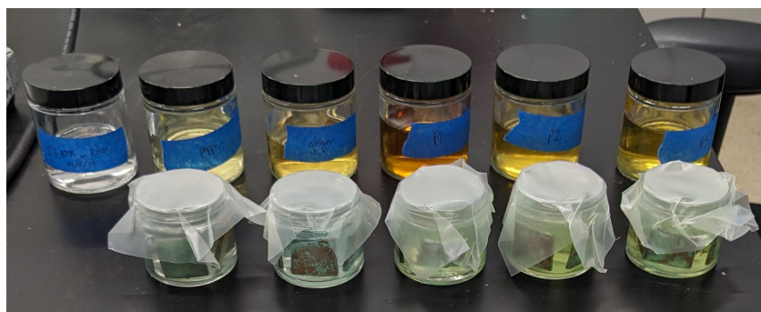
Figure A.22: Image detailing the immersion of all the coupons in inhibitor solution. From left to right: CG coupons immersed in pure ethanol, BTA-G coupons immersed in 3% BTA, P1 coupons immersed in 100 ppm of propolis 1, P2 coupons immersed in 100 ppm of propolis 2, and P3 coupons immersed in 100 ppm of propolis 3.
