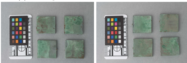
(b) BTA-G coupons after 24 hour immersion in 3% BTA solution
