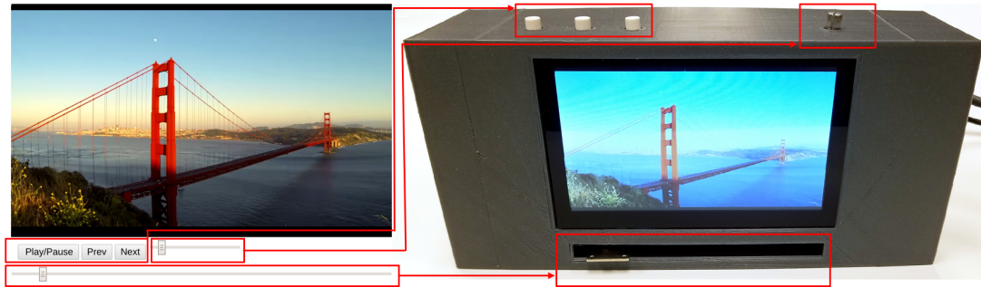
Figure 3.4. Video Player: At left, a demo of a video player which provides a familiar on-screen interface for playing videos. At right, Amalgam allows the same demo to drive a fully-tactile interface, the only difference being the style sheet.
