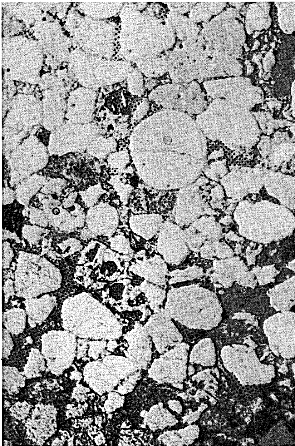
Figure 31. Sandstone, well M-96 at 1979 m depth. This is a fine grained, moderate to well sorted rock, with secondary porosity shown in a dot pattern. The grain in the center is a partly leached feldspar. View is 0.5 mm across.
