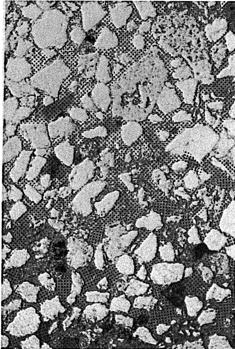
Figure 28. Photomicrograph of sandstone core sample from well M-20, at 915.3 m depth, plane polarized light. The dotted areas in this view are pores mostly resulting from removal of carbonate cement and feldspar. Elsewhere in this section, the cement is present. Measured porosity is 23.7% in this rock. View is 1.2 mm across.
