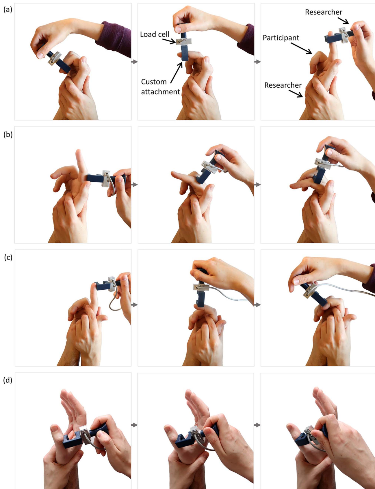
Figure 1. Custom load cell attachment used to move the participant's finger while measuring the force required to assist with the movement. Movements assessed were (a) index finger extension, (b) flexion of the metacarpalphalangeal (MCP) joint on the index finger, (c) flexion of the proximal interphalangeal (PIP) and distal interphalangeal (DIP) joints on the index finger, and (d) thumb opposition.
