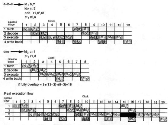
Figure 3: Pipeline Stall Example in SPARC.
