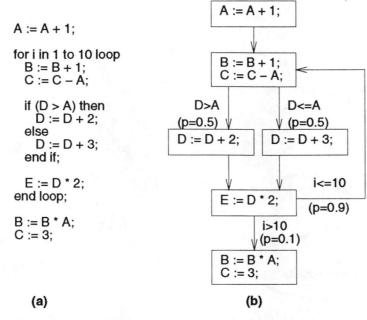
Figure 1: (a) VHDL program, (b) basic block graph.
