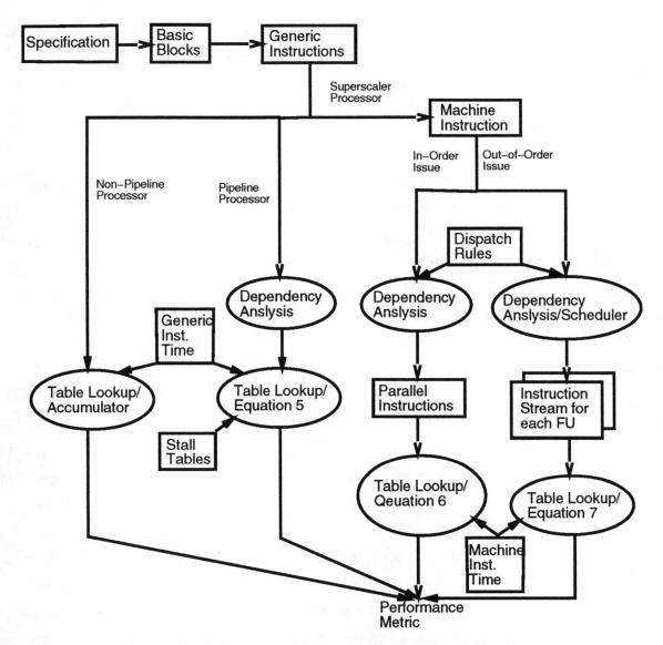
Figure 9: Software Performance Estimation Flowchart.
