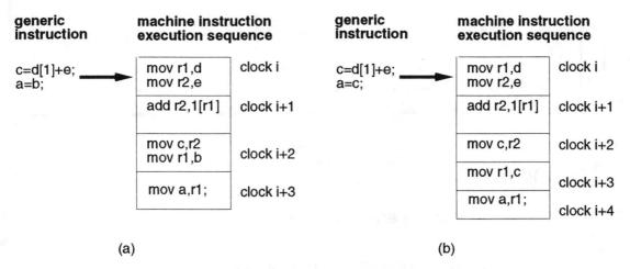
The estimation model of in-order issue superscalar processor was shown in Figure 6. This model adds a new feature: each function unit can handle more than one instruction.
