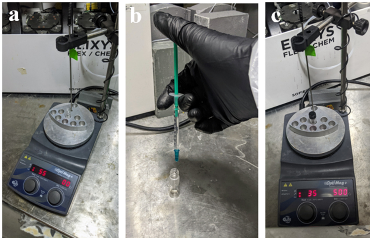
Figure 4.8. Photographs of the ^{18}\text{F} -deoxyfluorination protocol. A) Diethyl ether is evaporated at 55 °C (step 15); b) Peptide solution is added to the dried, ^{18}\text{F} radiosynthon (step 19); c) The reaction vial is sealed and heated to 35 °C (step 20). Photographs were taken in a hot cell but without the presence of radioactivity.
