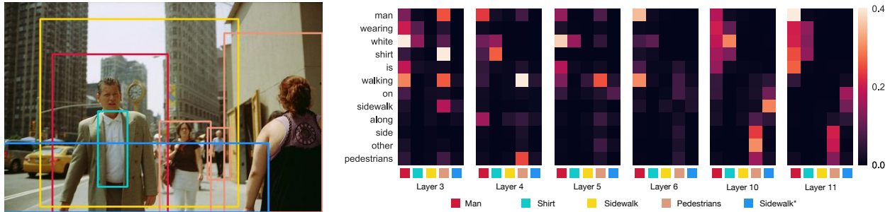
Figure 2.1: Attention weights of some selected heads in VisualBERT. In high layers (e.g., the 10-th and 11-th layer), the model can implicitly grounding visual concepts (e.g., “other pedestrians” and “man wearing white shirt”). The model also captures certain syntactic dependency relations (e.g., “walking” is aligned to the man region in the 6-th layer). The model also refines its understanding over the layers, incorrectly aligning “man” and “shirt” in the 3-rd layer but correcting them in higher layers.
