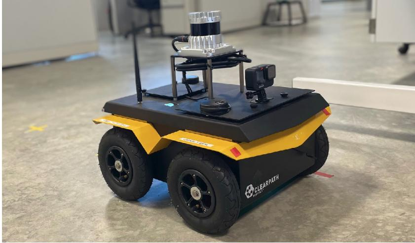
**Figure 4.9.** Jackal unmanned ground vehicle.
