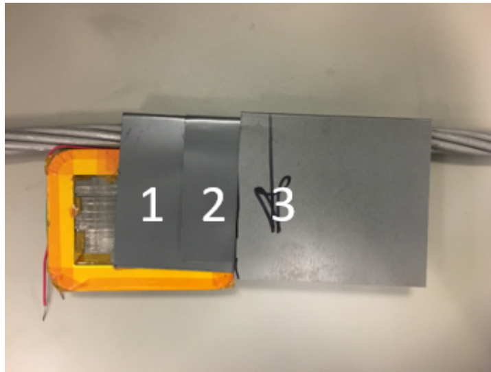
Figure 6.1: Energy harvester with up to three flux guides
