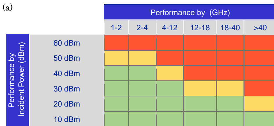
Figure 1.2 an illustrated review of P-I-N diode limiter performance, based on available products from one vendor, Microsemi [2]. The graphic highlights the typical constraints of commercial silicon P-I-N diode limiter function as a function of peak power and frequency. Green indicates good performance, red indicates poor or limited functionality
