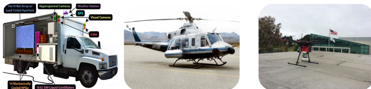
Figure 2.1: Representative detector platforms for comparison. (left) Lawrence Berkeley National Laboratory's (LBNL) Radiological Multisensor Analysis Platform (RadMAP). Source: [19] used with permission from J. Curtis and V. Negut. (center) The National Nuclear Security Administration's (NNSA) rotary-wing Aerial Measurement System (AMS). Source: [20] used with permission from P. Wasiolek. (right) LBNL's prototype Localization and Mapping Platform (LAMP) mounted on a small, commercial unmanned aerial vehicle (UAV). Source: [21] personal photograph.
