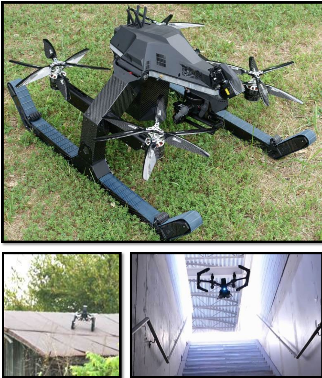
Figure 5.8: Pegasus III by Robotic Research (top) driving on land, (bottom left) perched on a rooftop, and (bottom right) flying up a stairwell. Source: [124] used with permission from J. Frelk of Robotic Research LLC.
