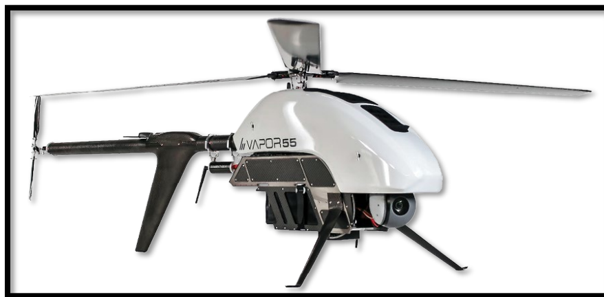
Figure 5.6: AeroVironment's Vapor 55, an example of a battery-powered unmanned helicopter. Source: [119] used with permission from B. Carraway of AeroVironment.
