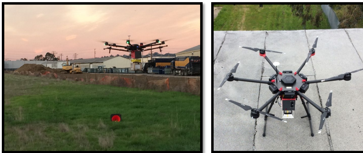
Figure 5.5: (left) Photograph of a DJI Matrice 600 Pro in flight with a prototype 3-D radiation mapping payload developed at the Lawrence Berkeley National Laboratory. Source: [139] used with permission from R. Pavlovsky. (right) The same platform with a different radiation detector payload on the rooftop of Bldg. 128. Source: personal photograph.
