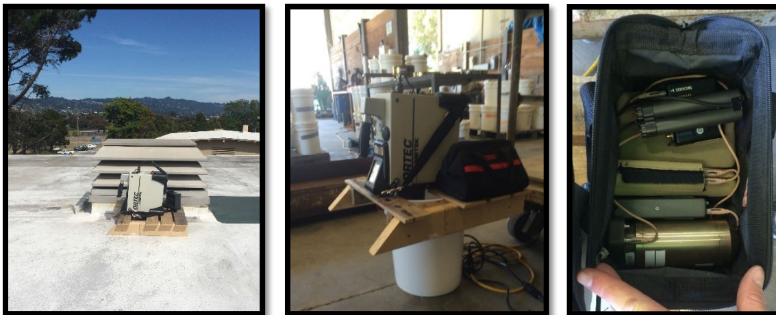
Figure 4.1 (left) An inverted ORTEC DX-100 high-purity germanium (HPGe) detector on an improvised stand. (middle) The HPGe detector raised from the floor with a bucket. (right) The contents of the bag include various prototype detectors on loan from the Defense Threat Reduction Agency (DTRA). Source: personal photographs.
