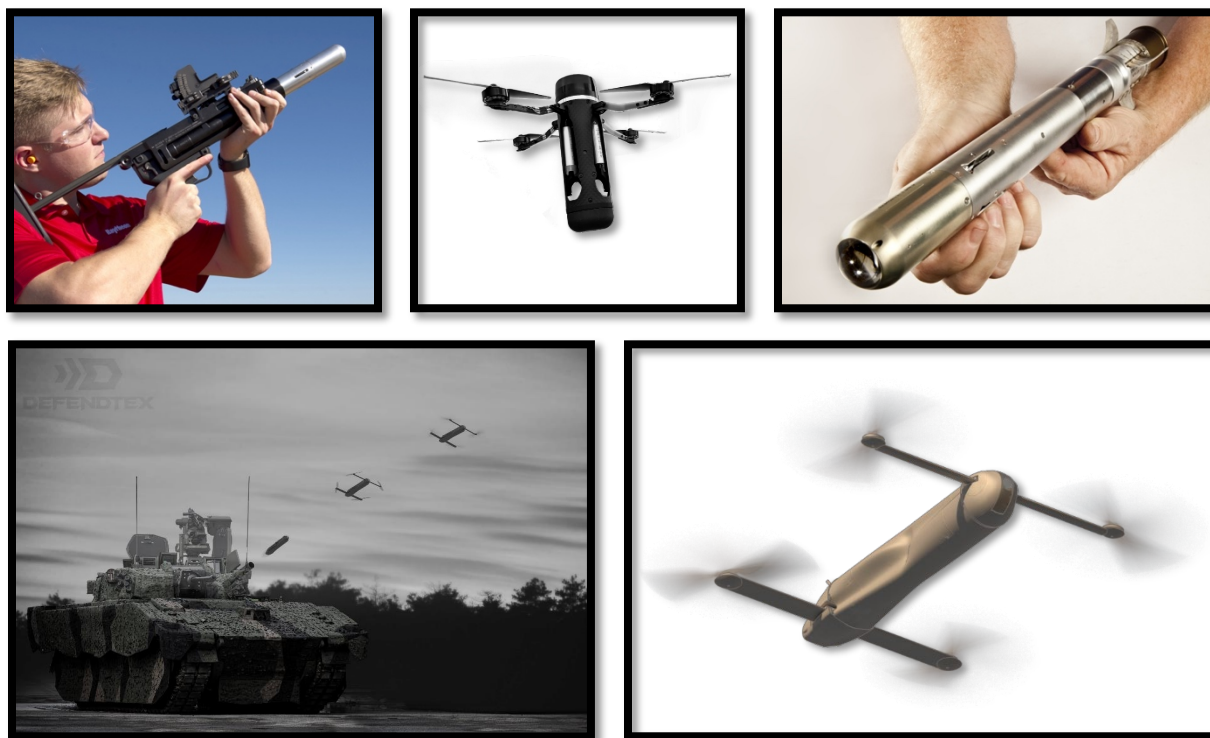
Figure 5.9: Examples of tube-launched projectiles and missiles that could deliver a detector payload to the target. (top left and right) The Pike® is a miniaturized, laser-guided weapon. Source: [125] used with permission from B. Edwards of Raytheon Company. (top middle) The Drone 40 Loitering Platform can be fitted with a small sensor payload. (bottom) The Drone 81 is in development with up to 1.1 kg payload, 45 km range, and 1.5-hour flight time. Source: [127] used with permission from T. Reddy of DefendTex.
