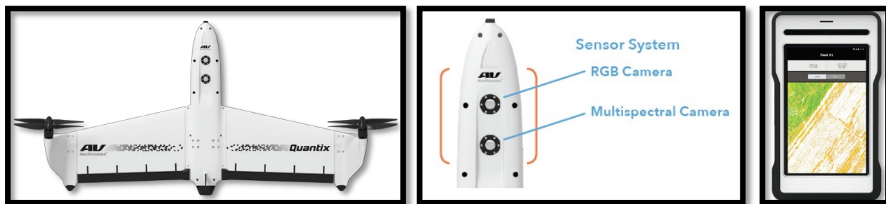
Figure 5.7: AeroVironment's Quantix, an example of a vertical takeoff and lift fixed-wing platform. This system is purpose-built for crop scouting and can cover 400 acres in a 45 m flight. Source: [142] used with permission from B. Carraway of AeroVironment.
